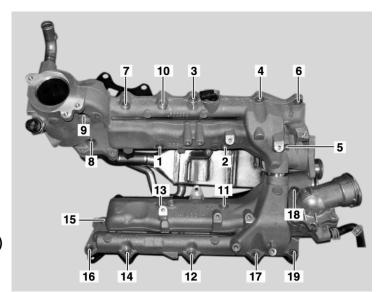
**18 Nm** Charge air distributor to cylinder head
